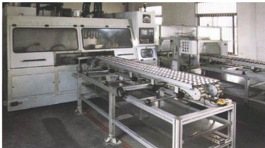
德国进口全自动双通道淬火机 Germany Imported Automatic Double Channel Quench Machine
