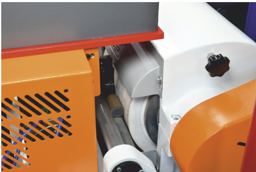
Fully automatic grinding of speed frame cots
