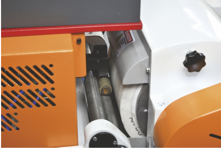
Fully automatic grinding of ring frame cots
